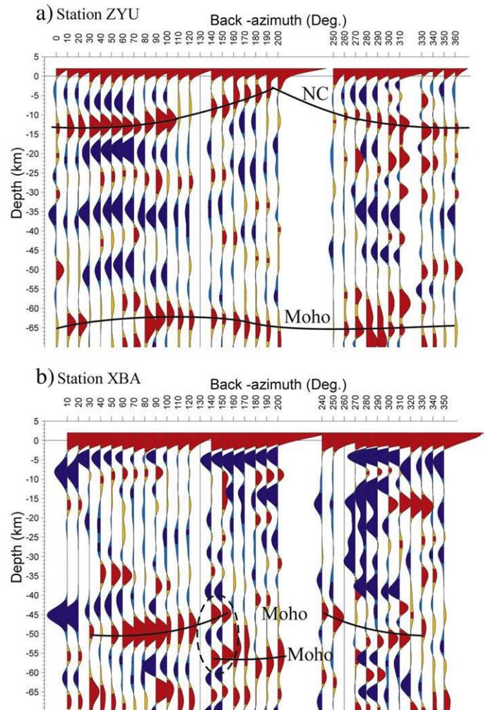
**Fig. 3.** Receiver functions stacked in 10° back-azimuth intervals at station ZYU (a) and XBA (b). The shallow north-dipping interface NC is observed at station ZYU. The Moho offset and double-pulse conversions (in the dashed circle) observed at station XBA. The delay time has been converted into depth with the CCP migration method.
