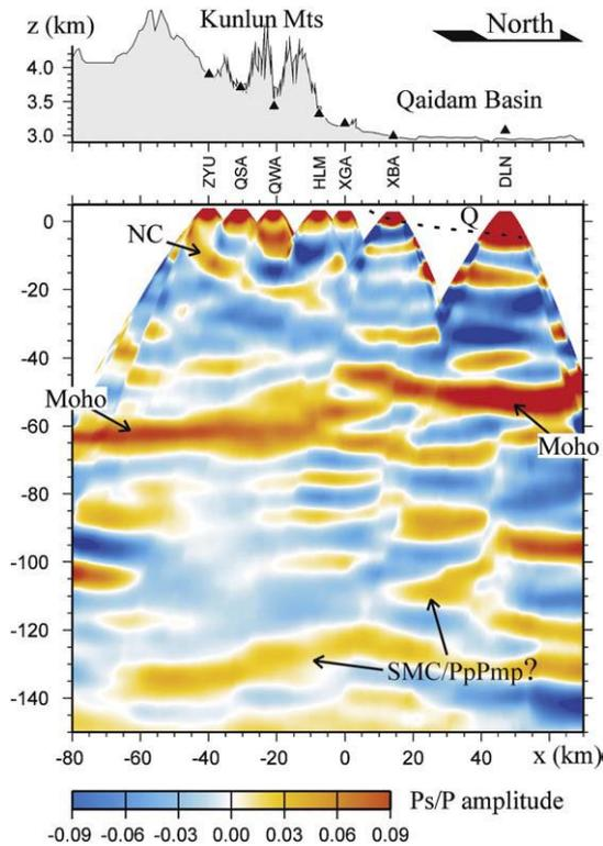
**Fig. 2.** Seismic image across the eastern Qaidam–Kunlun border constructed with radial P-wave receiver functions. RFs were back-projected and then stacked onto a north-south cross-section. The cross-section centered at station XGA (97.9307°E, 35.9417°N) and with the origin of the vertical axis at sea level. Top panel shows topography with station locations indicated by triangles. Color indicates the normalized amplitude of the converted phases.
