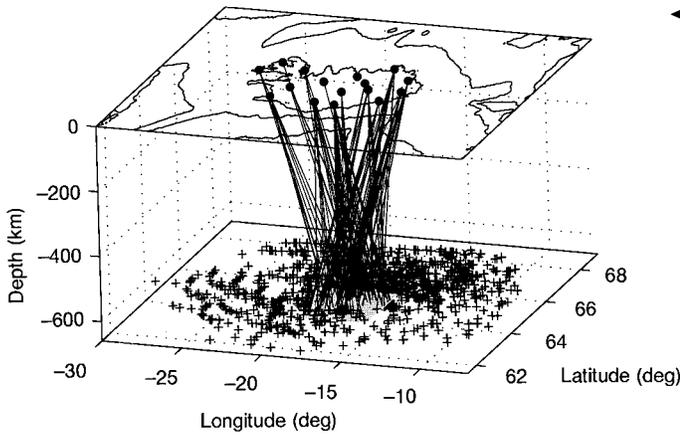
**Figure 2** The geometry of our experiment. Shown are the locations of the piercing points of P660s ray paths at the 660-km discontinuity (crosses) and the P660s ray paths (lines) from the central patch (grey square) to the ICEMELT seismic stations and the GSN station BORG (dots). The Icelandic coast and the Reykjanes and Kolbeinsey ridges are represented by regional bathymetry at 1-km contours. A total of 1,560 pairs of radial and transverse receiver functions sample the discontinuity.
