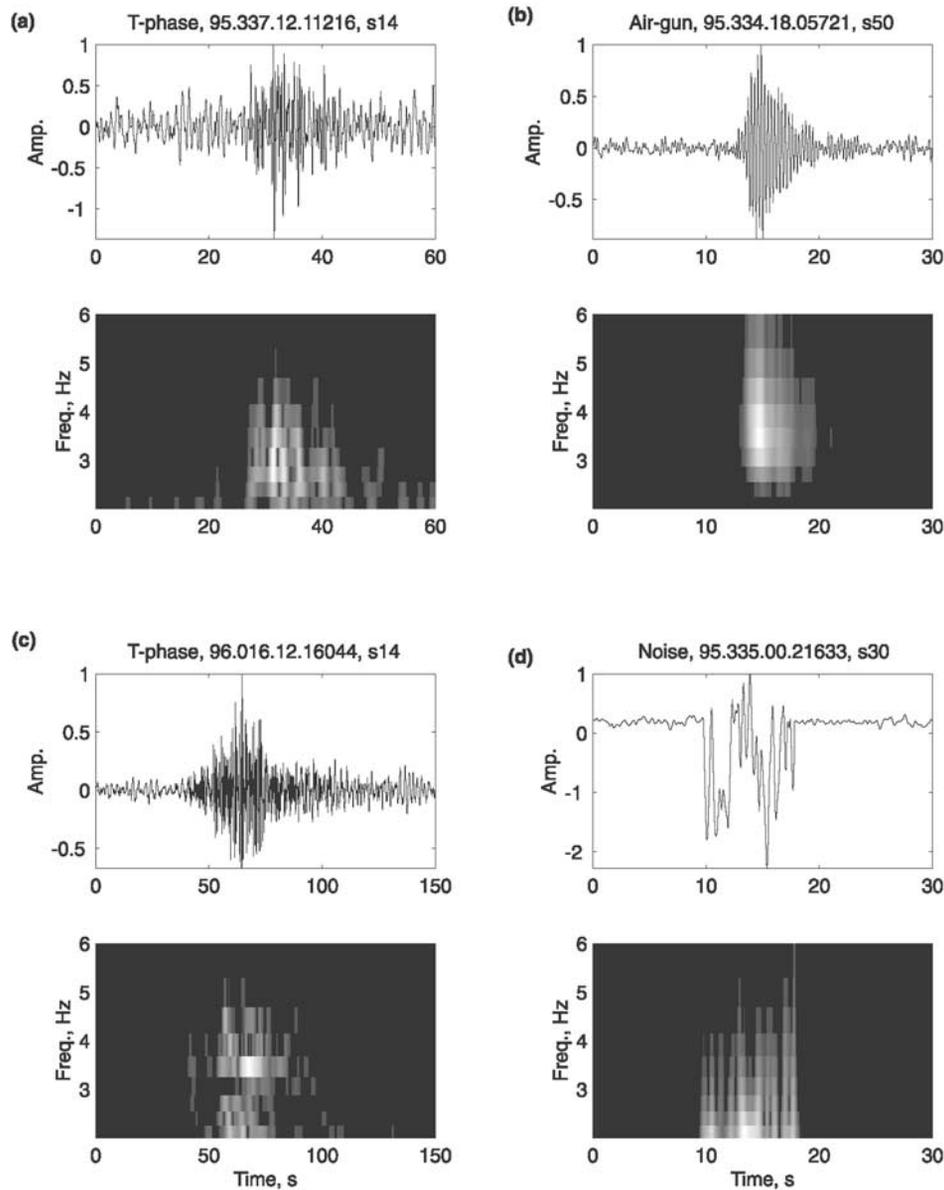
**Figure 2.** Waveforms and scalegrams of (a and c) two T phase events, (b) an air gun shot, and (d) an instrument noise burst.
