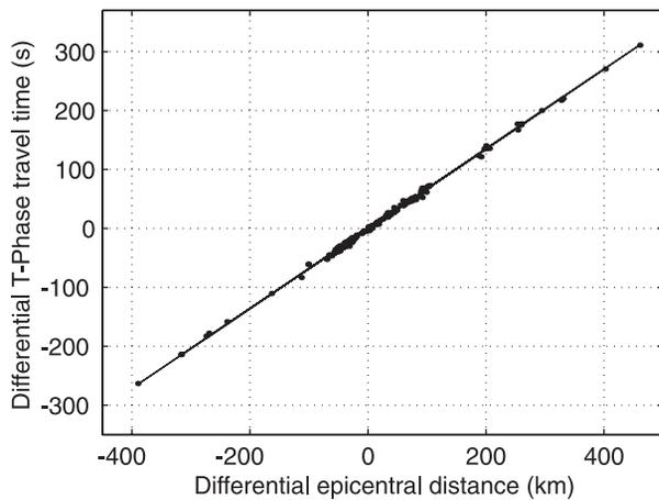
**Figure 5.** The least squares fit between differential T phase travel times and epicentral distances yields the T phase velocity.
