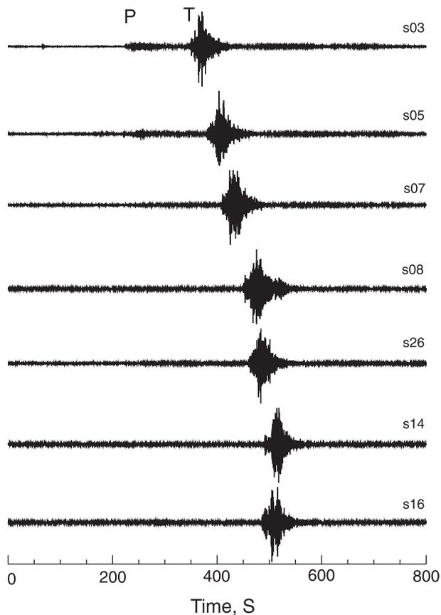
**Figure 4.** An example of regional earthquakes, as recorded on the vertical channel of several ocean bottom seismometers. *P* and *T* waves are identified.
