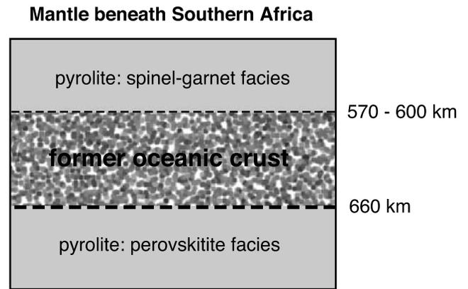
**Figure 3.** Schematic diagram illustrates a possible petrological structure of the mantle transition zone beneath southern Africa. Subducted oceanic crust accumulates at the base of the upper mantle, forming a  $\sim 70$  km thick layer with an upper limit near 570–600 km depth.
